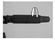
2. Move the gear shift lever quickly and firmly from neutral to reverse.
