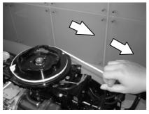
7. Give a strong pull straight out to crank and start the engine. Repeat it necessary.
