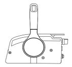
2. Tighten the steering friction adjuster by turning it clockwise to prevent the motor from turning freely.
