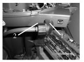
1. Water pipe plug; 2. Water pipe connector
