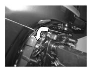
3. Loose the steering friction adjuster by turning it Counterclockwise, and adjust the steering friction according to operator preference.
