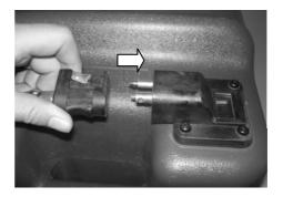
2. Connect fuel joints securely and squeeze the primer pump with the outlet end up until you feel it become firm (if equipped the fuel joint).
