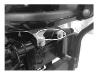
3. Disconnect the fuel line from the outboard motor.
